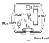
The wire coloured BLUE must be connected to the terminal marked N or coloured BLACK.
